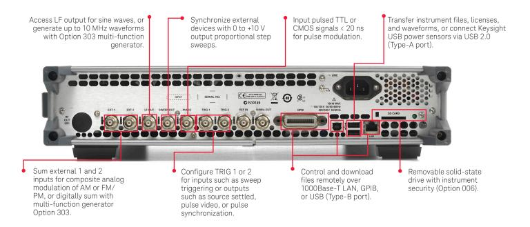
Note: The MXG and EXG X-Series analog signal generators have the same connector layout.
